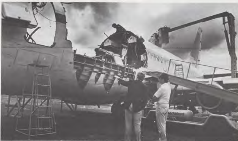
This high-time Aloha Airlines Boeing 737 lost an 18-foot section of its fuselage in April 1988, due to "significant disbonding" from the airline's failure to maintain and inspect the airplane properly. Looking over the damage are Joseph Nall (left) and Mike Benson of the National Transportation Safety Board.
