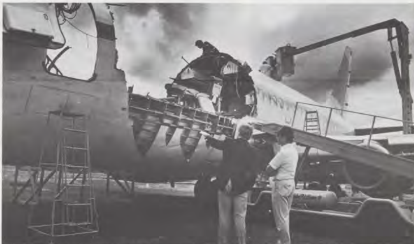
This high-time Aloha Airlines Boeing 737 lost an 18-foot section of its fuselage in April 1988, due to "significant disbonding" from the airline's failure to maintain and inspect the airplane properly. Looking over the damage are Joseph Nall (left) and Mike Benson of the National Transportation Safety Board.
