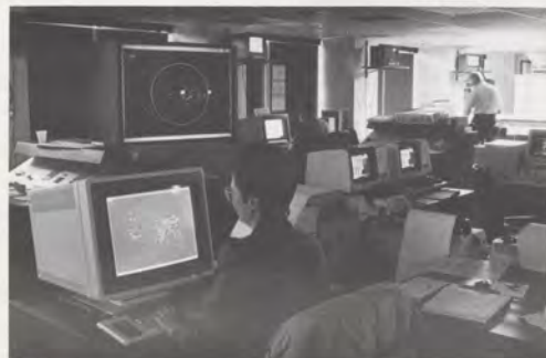
Traffic management specialist Debbie Compton operates an Aircraft Situation Display (ASD). Beyond is a large planning display, which may be used for a common additional screen. To her right are system performance monitors.
