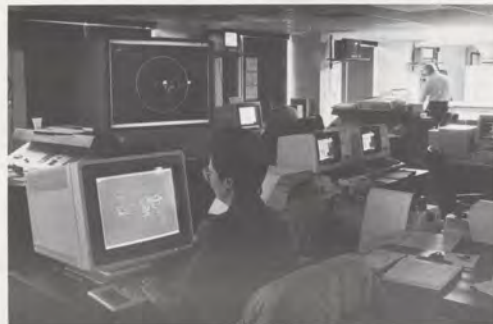
Traffic management specialist Debbie Compton operates an Aircraft Situation Display (ASD). Beyond is a large planning display, which may be used for a common additional screen.
