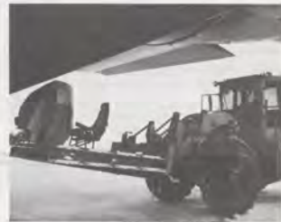
A forklift loads the palletized Sierra Portable Flight Inspection System aboard the Navy LC-130 Hercules being used for flight-inspection duty.
