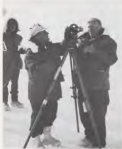
The author (center) and Christian Hafer (right) orient the theodolite to "Grid North" at the Williams Field TACAN site at McMurdo Station.
