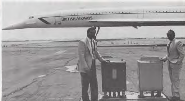
At each runway intersection being controlled are Stop Bar Remote Switching Units; a pair of which are shown here by JFK tower Manager Ed Trudeau (left) and Port Authority Aeronautical Services Manager Jack Gardner.
