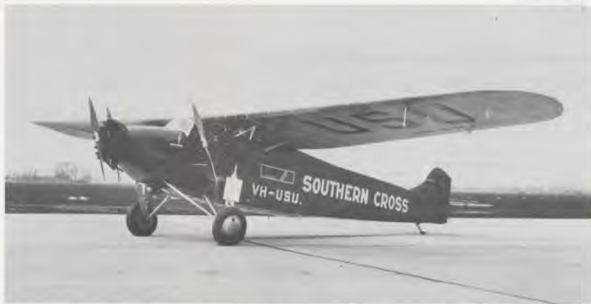
The Pacific-hopping Southern Cross carried wing tanks and a tank under the pilot's seat in addition to the main tank, for a total of 1,298 gallons of fuel.
