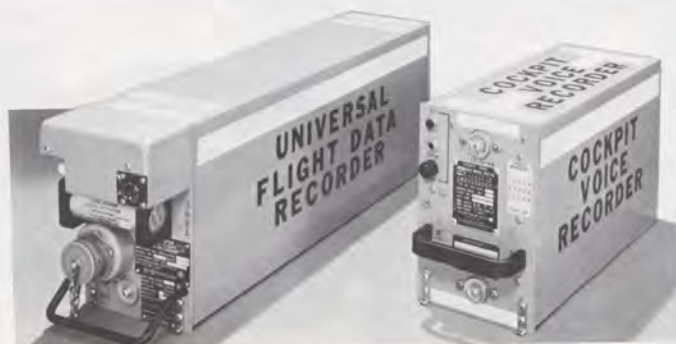
The flight data recorder and the cockpit voice recorder are mounted in the tail section of aircraft to minimize any damage to them on impact. Photo courtesy of the Sundstrand Corp.
