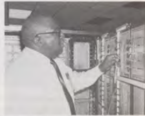
Diagnosing a problem in one of the storage elements of the IBM 9020 computer is Lawrence Hall, central computer complex electronics technician.
