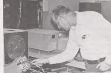
Electronics technician Howard Manning, from Covington's Knoxville, Tenn., Sector Field Office, aligns a BRITE scope.
