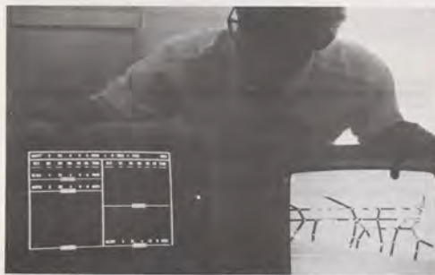
The two parts of The Airport Machine are the graphics display, which shows a departure lineup on taxiways of LaGuardia Airport, and the data display, which shows the same flights' identifications and arrival and departure times.
