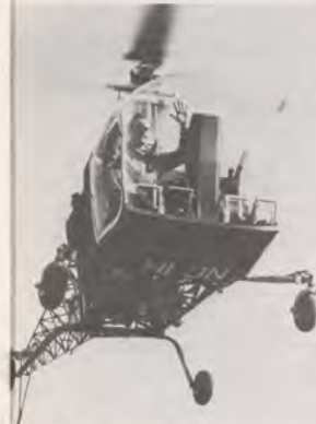
Bell Helicopter's chief pilot Floyd Carlson performs a hands-off stability test during the flight certification of the Bell Model 47—the first rotorcraft to receive Civil Aeronautics Administration type certification, 40 years ago on March 8. Its registration became NC-1H.
