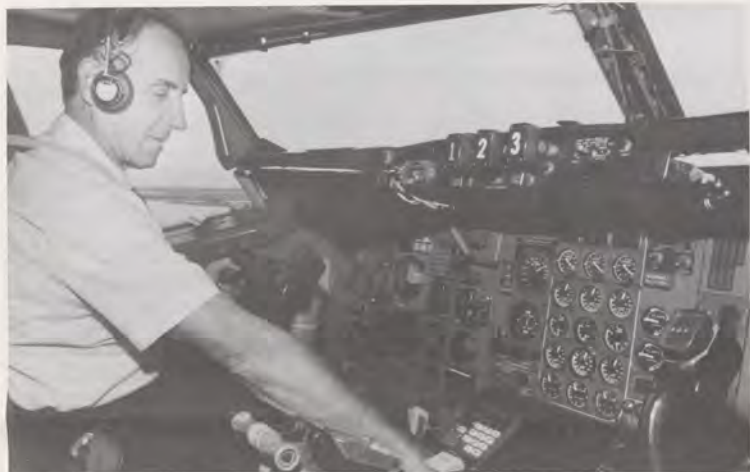
FAA chief test pilot Al Bazer adjusts the TCAS control panel aboard his Boeing 727 preparatory to flying a collision-avoidance test above the FAA Technical Center.
