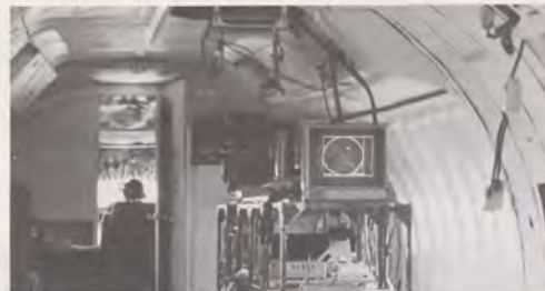
FAA's test Boeing 727 and its TCAS equipment in the forward cabin. Atop the racks is a display of TCAS III for an airborne technician to monitor. The spot in the center is the 727. An intruder is about three miles away at one o'clock. On the rack below is an engineering model of the TCAS III computer.
