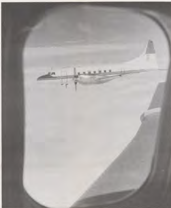
An FAA Convair 580 flies within 300 feet or less of the Boeing 727 to trigger alerts via warning lights, a radar display and lighted arrows and "eyebrow" lights on the vertical speed indicator.
