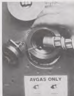
Fueling and fuel management are covered in the program. Here the emphasis is on using only the correct aviation fuel for the aircraft's engine.
