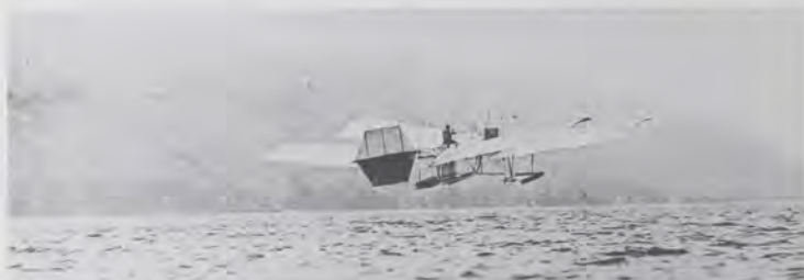
Langley's 1903 Aerodrome flew in 1914, but only after Glenn Curtiss modified and equipped it with one of his engines.
