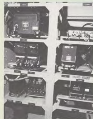
The flight inspection avionics for testing the ground nav aids.
