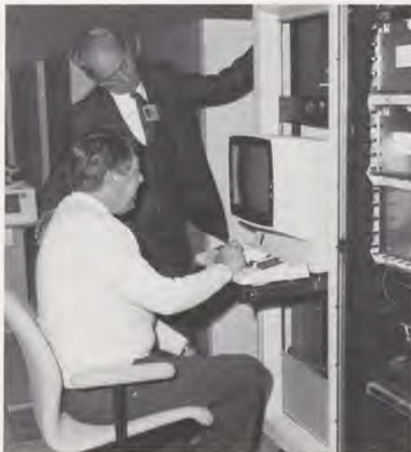
With System Evaluation Group's Bill Peters watching, Tony Clark of Air Traffic's En Route Field Support Section runs a routine on the Host's Processor Control Unit—a terminal for performing computer maintenance diagnostics.
