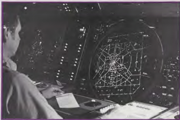
ARTS IIIA provides this Dallas-Fort Worth TRACON controller with alphanumeric data tags for all targets, beacon and non-beacon. Photo by S. Michael McKean
