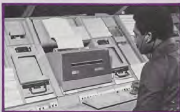
Computer update equipment (CUE) for flight data processing, shown here at the Memphis ARTCC, includes complete alphanumeric keyboard, flight strip printer and visual computer readout devices (on each side of the printer).
