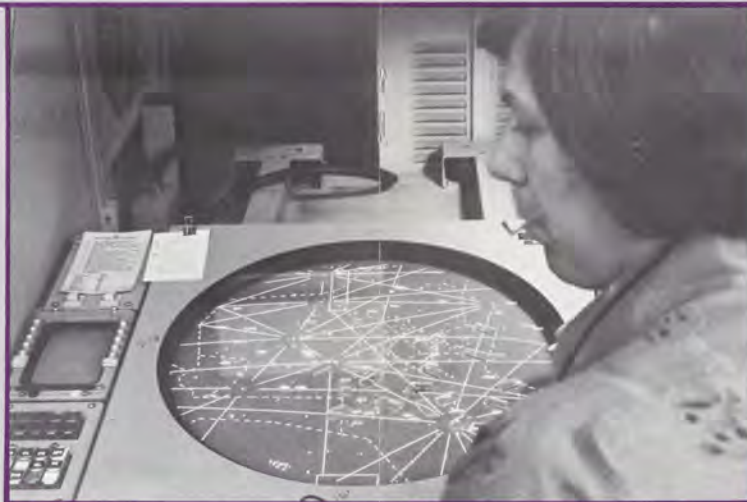
An enhancement to the Third Generation ATC System was Direct Access Radar Channel, a back-up system with limited alphanumeric and shrimp boats that now has been enhanced with full alphanumeric.
