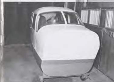
With the temperature at 25 degrees below zero and falling in a CAMI ice box cum wind tunnel, an FAA pilot seeks his survival gear inside a simulator.
