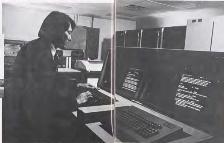
At the Cleveland ARTCC, George Krell, an E-Systems engineer providing contract support for FAA, operates the computer operator terminal console, which can monitor and interact with all the automated stations in the family.
