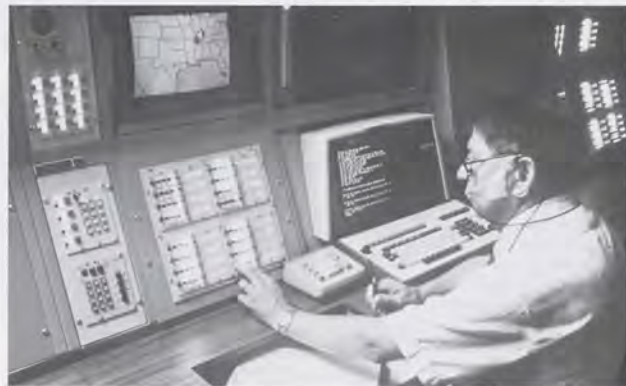
The Conroe, Texas, AFSS—part of the Houston "Family"—has already received its Model 1, but this earlier photo shows a combination of Service A equipment (at right), the new integrated circuit switching system and an element that won't formally be part of AFSSs until Model 2: a color weather graphics display (top), an interim replacement for closed-circuit TV that shows National Weather Service maps.
