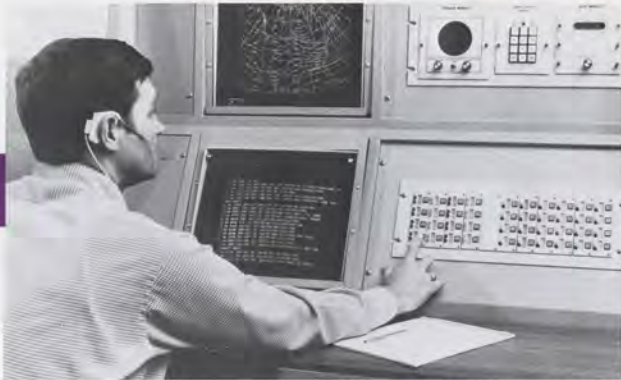
This could be 1988: an E-Systems mockup shows what a Model 2 automated flight service station position might look like, showing the Model 1 alphanumeric display and ICSS below and a color weather graphics display mounted above.
