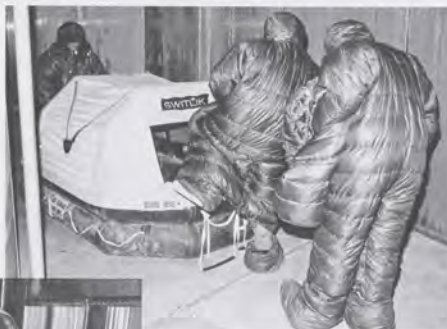
Dressed in insulated suits in the frigid arctic test chamber, pilots board a covered raft used as a tent.
