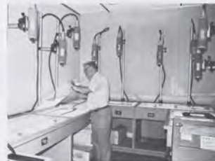
For the Model 1, Bridgeport specialist Richard Kniat positions facsimile weather maps under closed-circuit TV cameras that feed TV monitors at the pre-flight, in-flight and NOTAM Positions.
