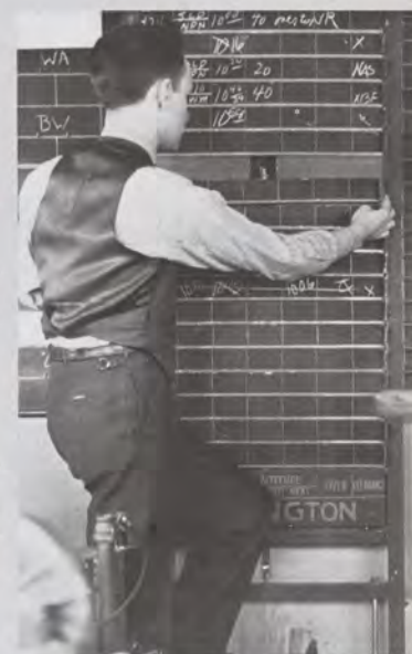
Controller Lee Warren operates his own design for the first ATC automation: A blackboard arrangement of slats that could be changed to keep flights in sequence. The pins at right anchored the slats. A foot treadle linked to pulleys raised the heavy column of slats below the one removed. It was a short-lived idea.
