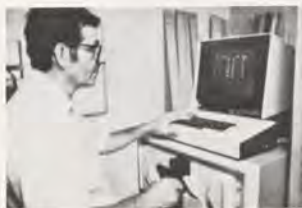
Electronics technician Ken Mitchell of the Boston Airway Facilities Sector used a display atop the LLWAS central computer unit to monitor sensor performance.
