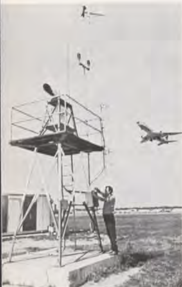
Electronics technician Wilbur Horton checks one of the earliest LLWAS sensors in a test at Atlanta International Airport. This boundary remote unit has the Fairchild configuration.
