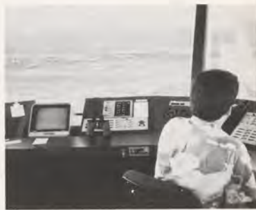
One of the local controller displays in the Honolulu Tower provides the controller with a LED display of wind speed and direction for each sensor and an aural alarm if wind variation exceeds 15 knots.
