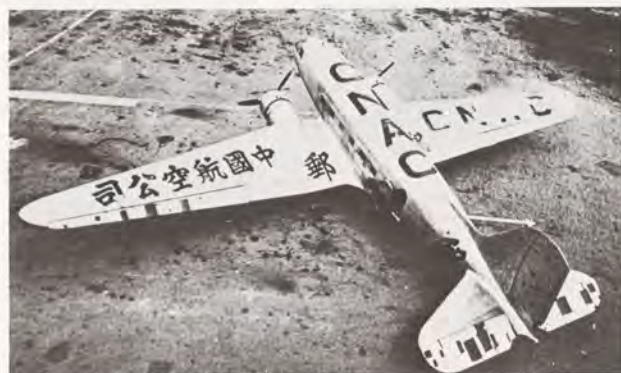
The legendary DC-2½ of the China National Aviation Corp. was a DC-3 fitted with a DC-2 wing after a Japanese bomb blew off its wing. It took a 12-degree setting of left wing trim to keep it level on its 900-mile ferry flight.
