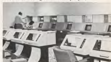
Jim DeBerry of E-Systems, Inc., and Sandra Mahlberg from the Chicago ARTCC help perform system shakedown of the Flight Service Data Processors (FSDP) at the Automated Flight Service Station position consoles and line printers at the FAA Technical Center. The FSDPs are now being installed at the Cleveland, Ohio, ARTCC to serve the Cleveland; Dayton, Ohio; and Bridgeport, Conn., AFSSs.
