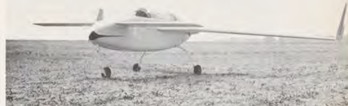
A Rutan Vari-Eze of the type involved in the save. It has a canard wing, winglets and a pusher propeller.
