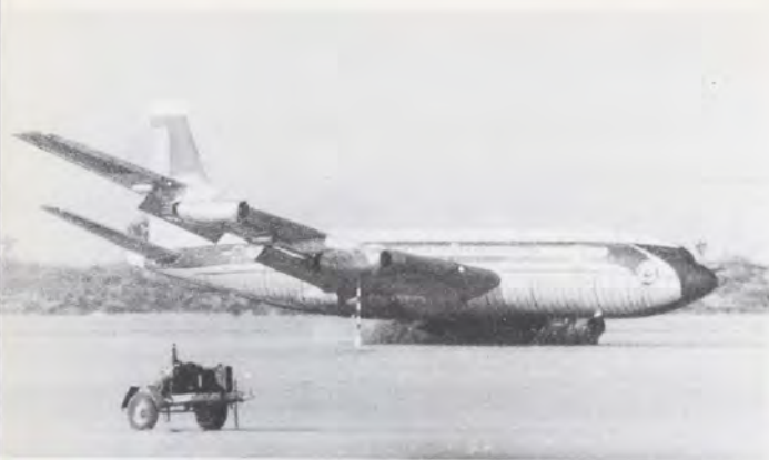
The FAA-NASA Boeing 720 raises a cloud of dust from the dry lake bed next to Edwards AFB as it lands wheels up as planned, but with its left wing low.
