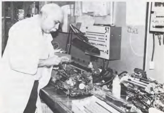
Peripheral device technician Harold Taubes adjusts a flight strip printer in the sector's repair shop.
