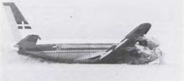
The aircraft skids 300 feet into the wing cutters (one appears just in front of the nose), which are designed to ensure fuel spillage for the AMK test.
