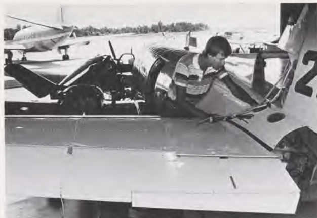
Southern Illinois University student Steve Hawkins checks the routing of control cables in an aircraft's tail section.
