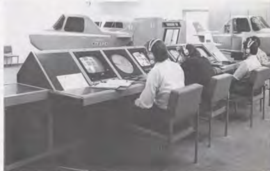
At a Link Trainer monitoring console, Embry-Riddle instructors watch trainer cockpit panels and a dial showing course headings during IFR training. Through a communications hookup, they can act in the role of air traffic controllers.
