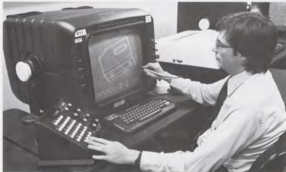
Computer technology is aiding design and manufacturing. Here, a McDonnell Douglas engineer uses a light pen as an entry device to modify the specifications of a part.
