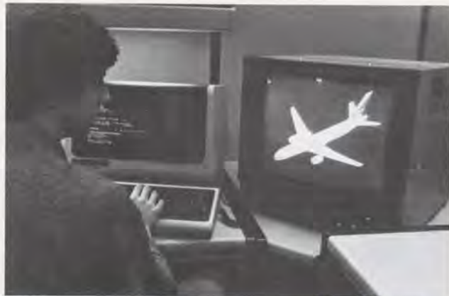
A Boeing Company engineer uses a computer imaging system to assist in aircraft design, an approach that could lower engineering design costs as much as 30 percent.
