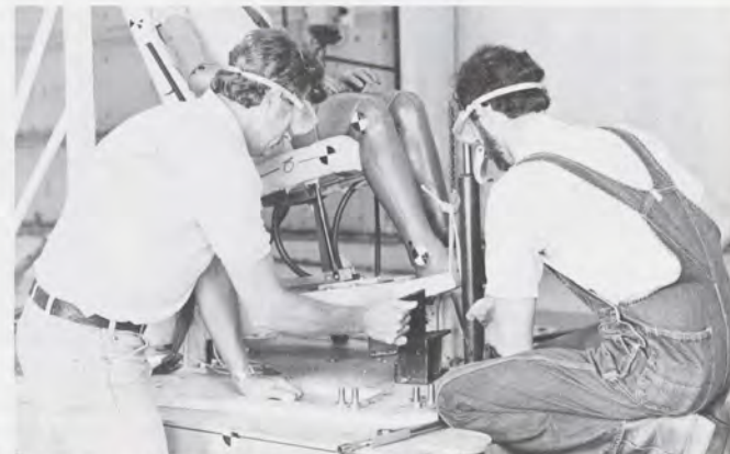
John LeGrange (left) and Dick Forsythe raise the pilot's seat to simulate a 10-degree deformity of the aircraft floor, supposedly bent on aircraft impact.
