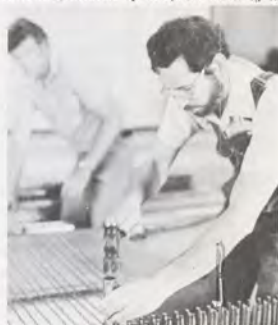
Dick Forsythe, engineering technician, installs a brake wire system, which stops the sled on which a test seat is mounted. The sled is pulled by a 5,500-pound weight.
