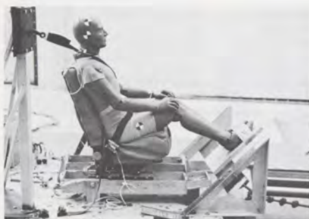
For a test run of two seconds, getting the anthropomorphic dummy test bed set up completely takes about four hours.
