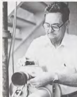
Photographer Lee Forest checks the 1,000-frames per second HYCAM camera that records the sled's impact in slow motion.
