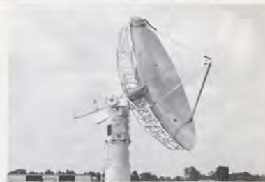
This 30-foot parabolic antenna is part of FAA's weather radar test bed for both terminal and enroute use. The installation is at Olive Branch Airport, 10 miles from Memphis, Tenn., International Airport.
