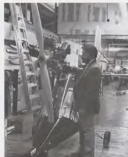
Following a static load test on a Pioneer ultralight, inspector Ness checks it over for deformation.
