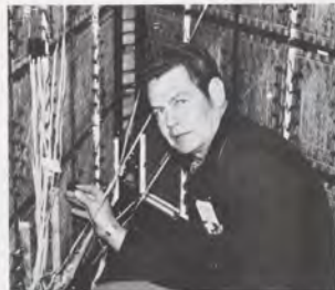
Bob Hutchins, central computer complex technician in the Flight Data Processing Unit, attaches logic analyzer probes to the compute element 1 of the IBM 9020A.
