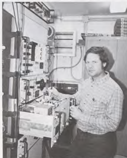
Electronics technician Fred Roath performs maintenance on a Cardion distance-measuring equipment (DME) drawer in Dillingham, Alaska, Sector Field Unit.
