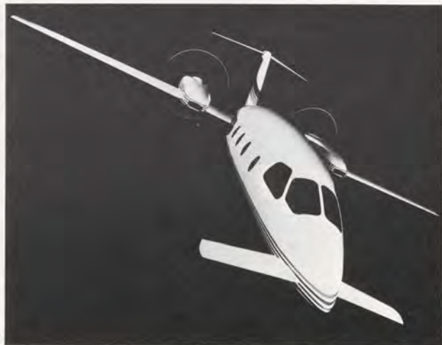
This full-scale mockup of the Gates-Piaggio GP-180 shows a canard control surface at the nose and air intakes denoting the turboprop engines. The company claims 400-knot speed, 2,100-nautical-mile range, 41,000-foot ceiling and fuel efficiency of 1 nm per pound.
