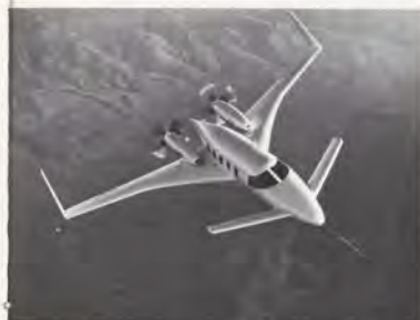
Also a 400-mph pusher turboprop with a canard is Beechcraft's Starship 1, which also carries drag-reducing winglets.
