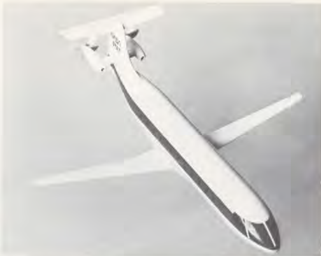
This model of a commuter aircraft at NASA's Langley Research Center combines propfan-equipped turboprop engines with natural laminar flow control and a high-aspect-ratio wing for high fuel efficiency.
