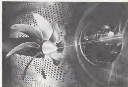
The thin-bladed, swept propfan under investigation by NASA holds the promise of delaying compressibility effects of propellers and the attendant drag rise and the noise-producing supersonic shock waves and vibration. This would permit reducing aircraft insulation and fuel use.
