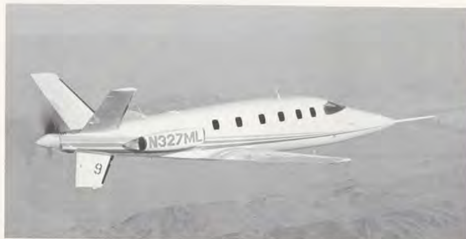
This was the first production prototype of the Lear Fan, a graphite-epoxy-composite-skinned turboprop that has the prop separate from the jet nacelle.
