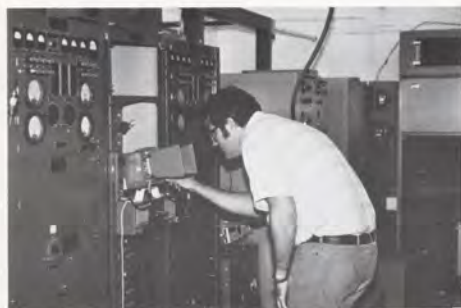
Electronics technician John Nimmo checks over the operation of the Scottsbluff VORTAC on an oscilloscope.
