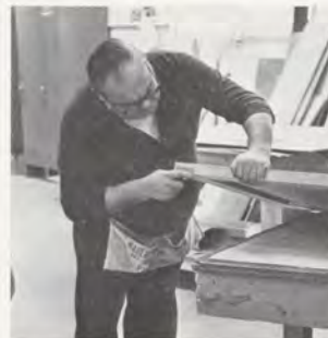
Charles Kuck reworks the laminate on the built-up edge of a table top.
