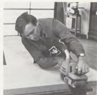
Joseph R. Smith uses a belt sander on a countertop to be laminated.
