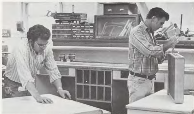
Clifton Bailey (left) planes a joint on a countertop bullnose and Jack Berry works on a drawer for a desk unit for the Technical Center's scheduled airline ticket office.
