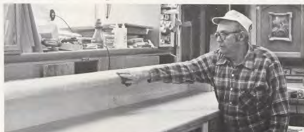
Painter Charles A. Smith wipes a project with a tack rag prior to painting.
