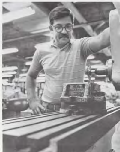
Dave Kennedy uses a horizontal mill for fabricating output connectors and an RML crystal holder.
