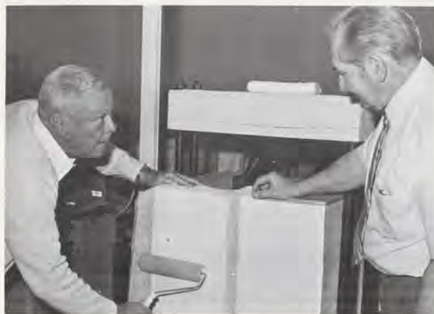
Gordon Ferris (left) applies glue to a gauze backing on the spines of stacks of the NAS Plan "Brown Book" on a wine press he donated. Watching how his car jack was used is dispatcher George Strigh.
