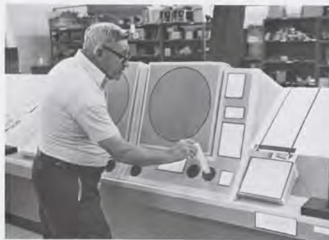
Cabinetmaker Milan May, who built most of the console, demonstrates how controllers will drop flight strips down a tube to the O'Hare TRACON below the cab.
