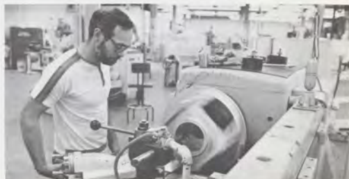
Dave Schneider, a machinist, repairs a part for an ARSR-1 rotary joint.
