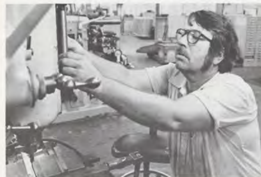
Machinist Glenn Reeves adjusts his milling equipment for fabricating an obsolete part for a long-range radar.
