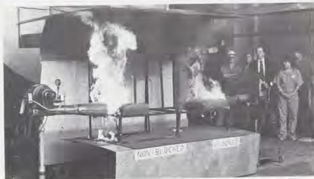
In a demonstration of ongoing fire safety studies at the FAA Technical Center, an ordinary, non-blocked airliner seat and one incorporating a blocking layer around the foam cushions were set afire. The blocked seat took longer to ignite.
