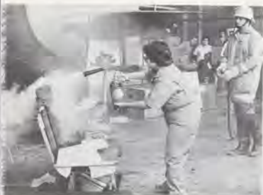
With a fireman in readiness as an extra measure of safety, a Tech Center employee uses a carbon dioxide extinguisher on an airline seat fire.
