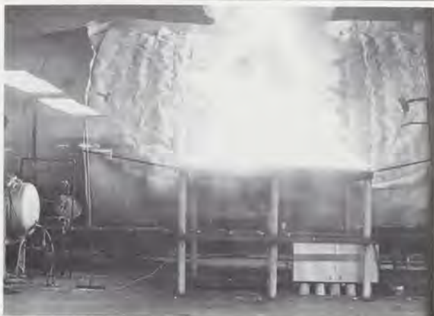
A C-133 fuselage is used to test the flammability characteristics of cabin interiors. Here, a table with a pan of fuel is ignited in front of an open door under a controlled wind to test cabin materials.
