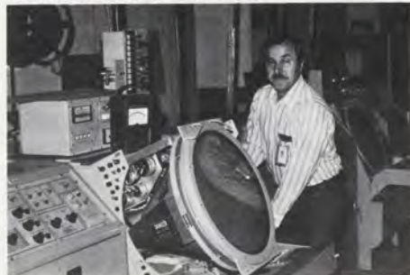
ARTS technician Joseph Hock works on the innards of one of the New York TRACON's radar scopes.
