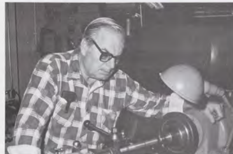
Machining a shaft for a gear box that will operate hangar doors at the Flight Operations Building is Albert Colwell.
