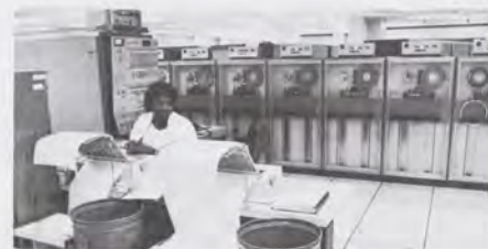
The National Airspace System IBM 9020 computer will soon be replaced with a new high-technology host computer.
