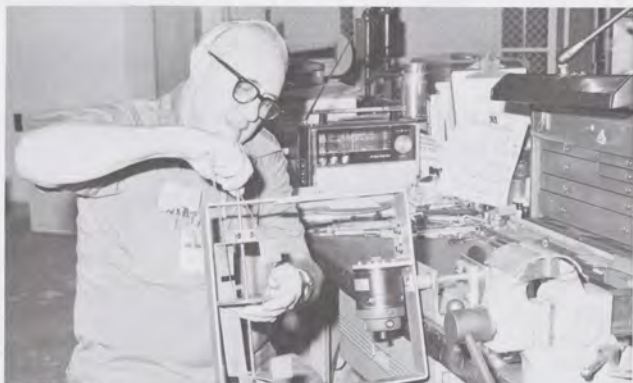
Bob Shinn assembles a device for a horizon simulator that will be used on the center's general aviation trainer (GAT-II).
