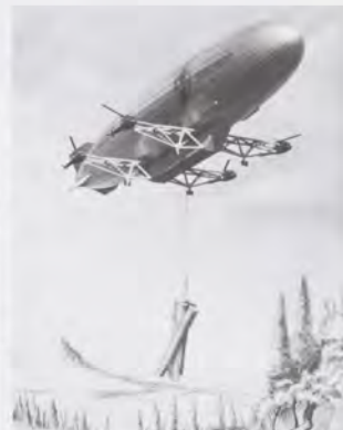
An artist's rendition of the hybrid Piasecki Heli-stat being developed under a Navy-Forest Service contract.
