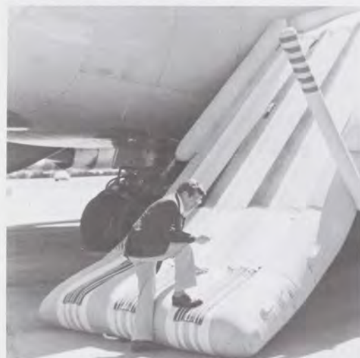
Assistant principal air carrier maintenance inspector Robert Sanchez looks at a door exit slide that failed during a test.
