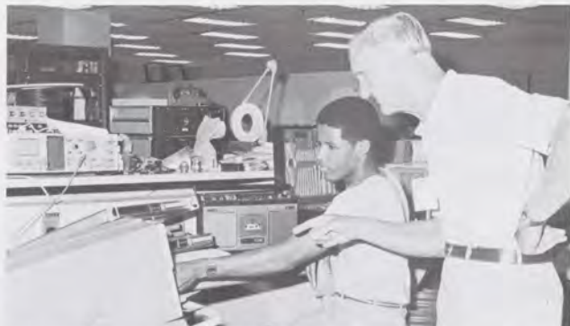
Tech Center meteorologist William Lewis checks 15-year-old Maurice Johnson's procedure in using an oscilloscope to set the level of a time signal from an aircraft tape recording during a storm.
