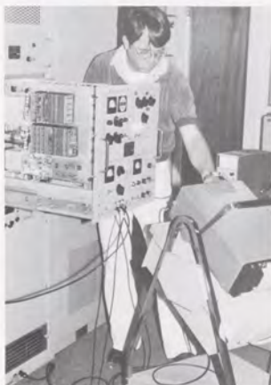
Electronics technician Ron Oberlercher checks waveforms on an air traffic control beacon interrogator.
