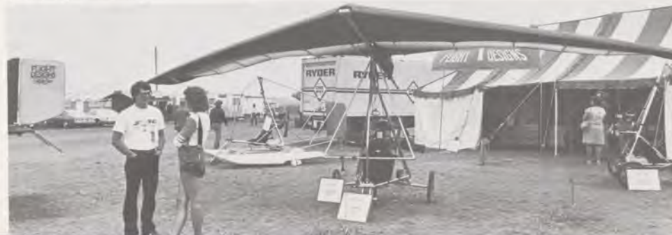
Flight Designs' Jet Wing (below) has a conventional delta wing like a hang-glider and is flown either as a hang-glider or a powered ultralight.
