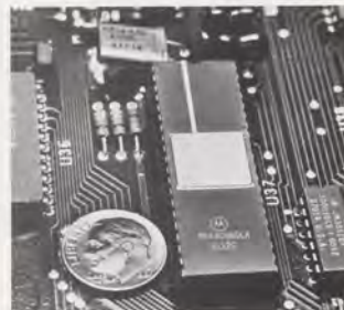
A microprocessor integrated-circuit module containing a large silicon chip is compared to the size of a dime. The circuitry in the chip is perhaps equivalent to that found in about 50 TV sets.
