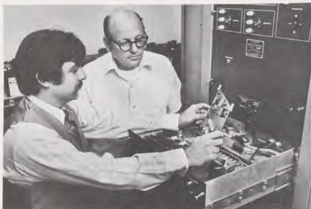
After making a fault diagnosis, instructor Don Torchio shows student/technician Bob Teseny, Enfield, Conn., the simplicity of unplugging a defective circuit board in the goniometer drawer of a VOR unit.
