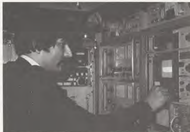
David Lantzy, Great Lakes communications specialist, tunes in a frequency on his SCAM van's spectrum analyzer to check the accuracy of a navigational aid.
