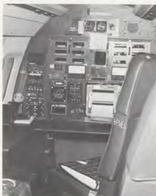
Improvements to flight inspection include the Automated Flight Inspection Computer System, now installed in 15 Sabreliner 80s and five Jet Commanders.
