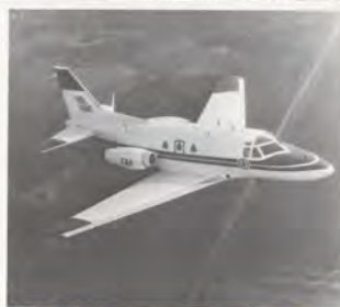
An FAA flight inspection Sabreliner 80. Replacement with turboprop aircraft to save on fuel is in the cards.
