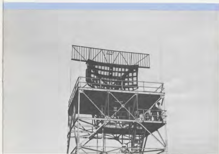
The newest terminal radar beacon antenna, which will serve Mode S in tomorrow's system, is a five-foot open array atop an ASR-8, here at Miami International Airport.
