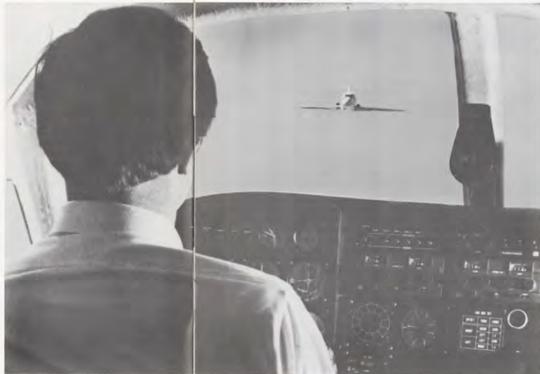
Two FAA Technical Center aircraft—a B-727 and a Convair 580—really fly at each other deliberately to trigger collision-avoidance equipment installed in their cockpit panels.
