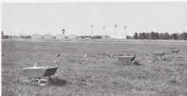
Four PAPI units are lined up at Teterboro, N.J., Airport to test the British glideslope system in a general aviation environment.
