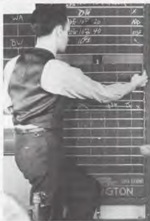
Controller Lee Warren operates his own design for the first ATC automation: A blackboard arrangement of slats that could be changed to keep flights in sequence. The pins at right anchored the slats. A foot treadle linked to pulleys raised the column of slats below the one removed.
