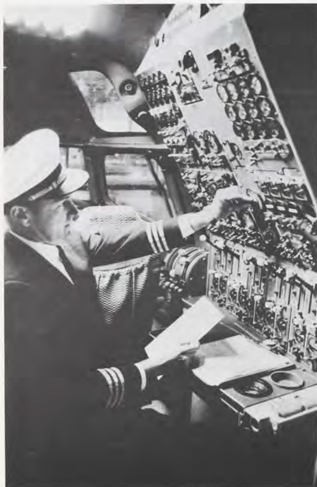
By 1961, the flight engineers handled instrument monitoring not servicing functions, such as this one aboard a DC-8.
