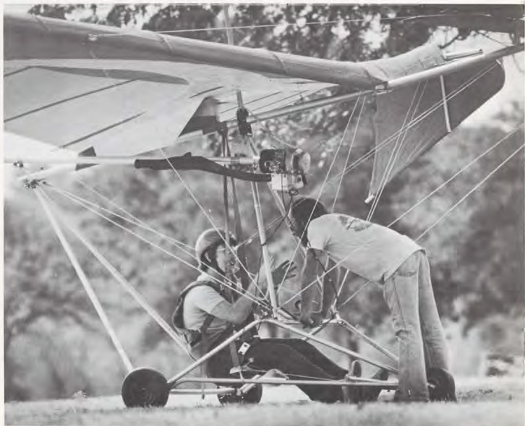
Pilot Jim Poyner discusses a completed training flight with Lone Star Owner Gary Scheer. The Eagle features "dragelons" on the wing tips that function as rudders.
