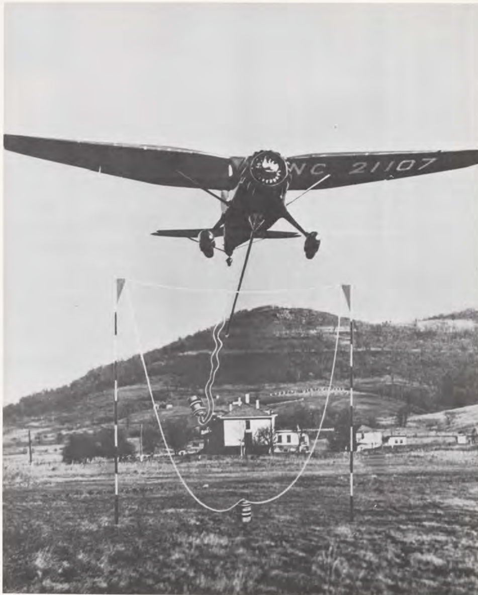
An All American Aviation Stinson Reliant drops the mail in an open field as it prepares to hook an outgoing canister.
