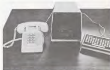
A VuSet CRT acoustically coupled to a push-button telephone will be able to retrieve alphanumeric data from the FSS computers, as well as display a digital map weather radar summary, such as the one shown at the top for the Houston, Tex., area.
