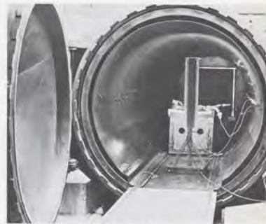
An epoxy-laminate part is ready to be cured in Lear Fan's giant autoclave under high heat and pressure.
