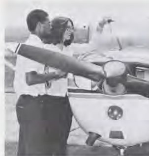
Pilot safety begins at the beginning with the walk-around. Embry-Riddle instructor Nigel Lemons and Tech Center employee and student pilot Roberta Crosson check a Cessna's oil level.
