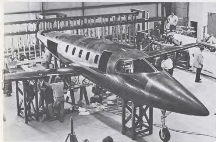
A prototype for demonstration purposes is assembled with some riveting to hold the epoxy-bond panels in place while being cured, in lieu of the tooling needed for an epoxy-only bond. For certification, the prototype will only be bonded.
