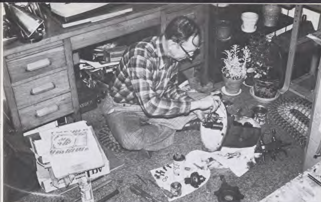
John "Cadillac" Smith reassembles the rebuilt transmission for his 1940 Ford.
