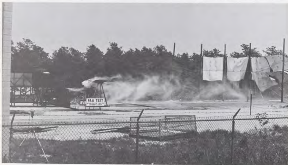
Standard aviation fuel spilled from a wing section and ignited at the FAA Technical Center's Wing Spillage Test Facility goes up in a huge fireball. (top)
