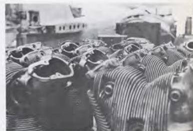
Rows of radial-engine cylinders wait in a workshop for reinstallation in a World War II Japanese Nakajima "Irving" being restored by Smithsonian craftsmen.
