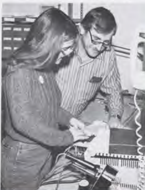
Technicians Maura McGrath and Joseph Hock repair an ARTS IIIA keypad.
