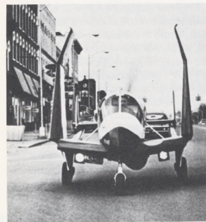
Two more-recent entries in auto-plane design around 1973 were the AVE Mizar (top), a combination of a Ford Pinto and a Cessna Skymaster, and the home-built Bryan III, its wings folded for driving around Highland, Mich. Both were subsequently involved in fatal crashes.
