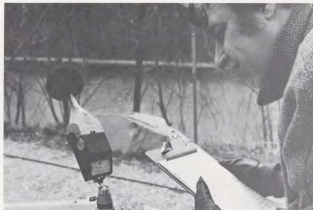
Part 36 of the FARs came in just ahead of the '70s. An FAAer takes measurements of the decibel level of Washington National takeoff traffic with an audio meter.
