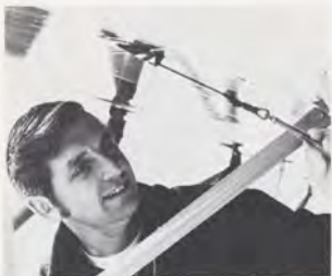
Seattle maintenance inspector Alan Butterworth inspects a control-cable turnbuckle on an amateur-built aircraft, an ongoing job to ensure flying safety.
