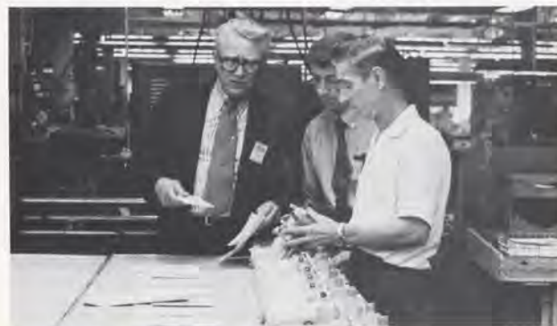
A manufacturing inspector discusses the match-up of passenger door motors with their specifications with the manufacturer's assembly line inspectors.
