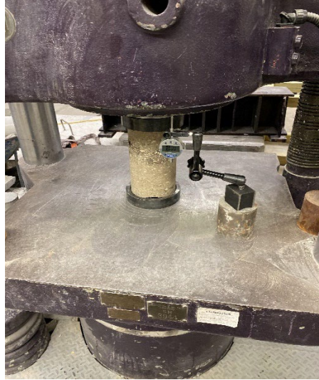
Figure 3.2: CTB Elastic Modulus Test Setup
