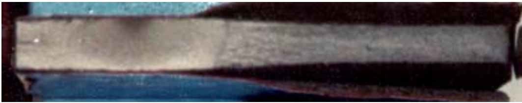
Figure 3.29 Surface failure of Specimen WD-3
