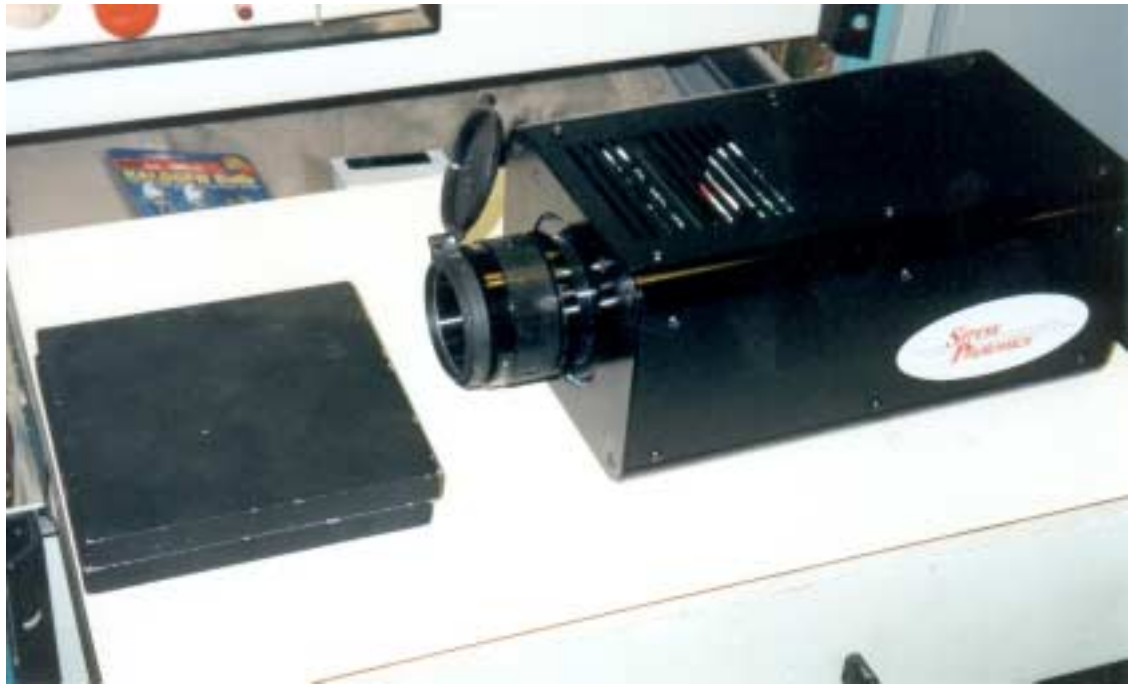
Figure 3.34 The IR camera and calibrate plates
