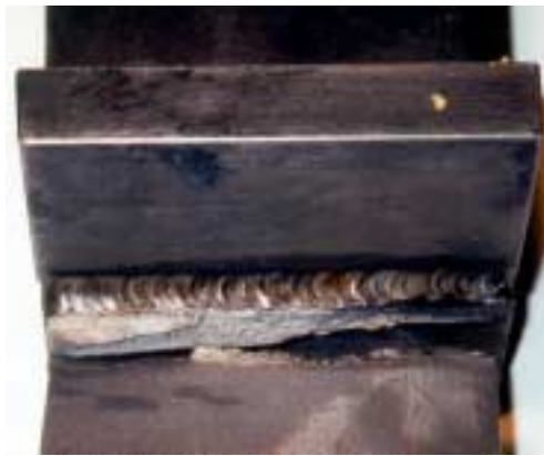
b) Front view of failed specimen
